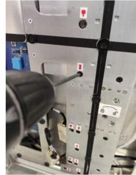
Uninstall 16 pcs M4 flat head screws
